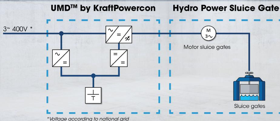
To ensure the emergency operation of the AC motors, UMD™ system secures operation of the AC-motor from both the mains and battery supply.
